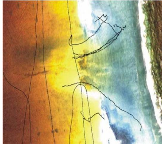
Figure 9: Flow over Rongelap reef flat, particle tracked with GPS.
