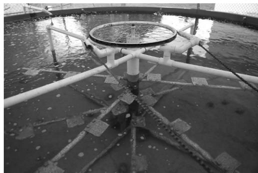
Figure 1: The Coral-sel in position at the UM Aplysia Resource Center. Each attachment site bears experimental plates at positions 15, 50, and 85 cm from the axis of rotation.
