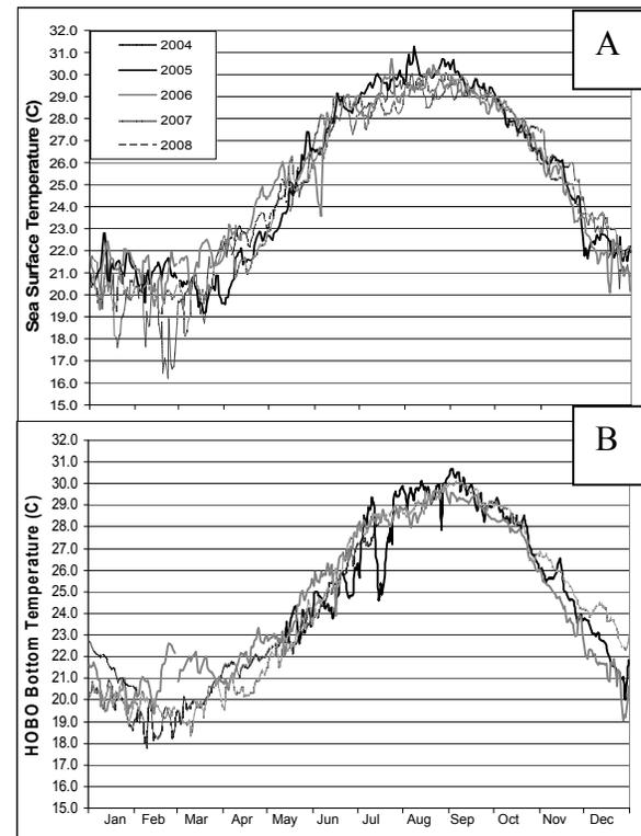
Figure 4: Average daily temperatures from 2004 – 2008. (A) Sea surface temperatures from NDBC Buoy 42019. (B) Bottom temperatures from the surface of Stetson Bank (23.5 m depth) from HOB0 temperature probes.
