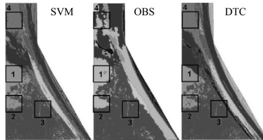
Figure 3. The final classified surfaces developed from the MBES imagery using SVM (left), OBS (middle) and DTC (right). Areas 1, 2, 3 and 4 denote locations where the classified results did not meet one or several of the qualitative accuracy criteria as outlined above.
