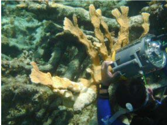
Figure 2: Spectral measurements collected of elkhorn coral ( Acropora palmata ) using the GER 1500 spectroradiometer in underwater housing.
