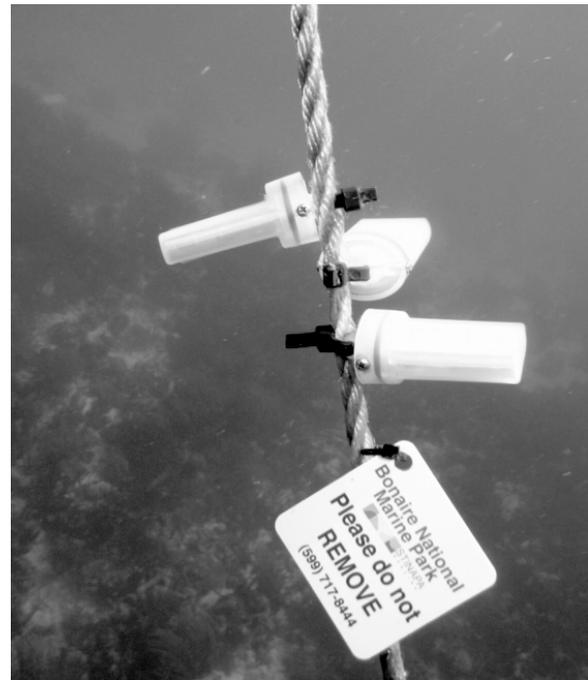
Figure 2: LMSP Rainbow Sensor Array on a mooring line in the Bonaire National Marine Park.
