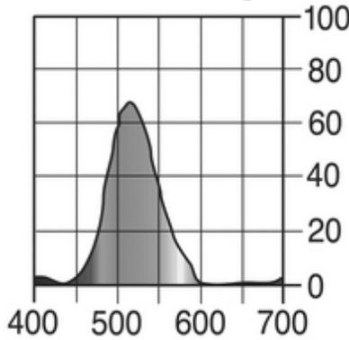
Figure 4: Filter transmission spectrum for Lee Filter #124, Dark Green (<http://www.leafilters.com/>). The x-axis and y-axis are the same as in Figure 3.
