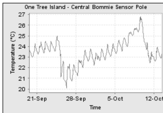
Figure 4. Plot of temperature over time for the bottom (lagoonal) sensor on the sensor pole located in Central Bommie, One Tree Island lagoon, southern Great Barrier Reef for late September 2008.
