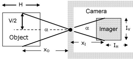
Figure 2: Basic optics of a CCTV camera
