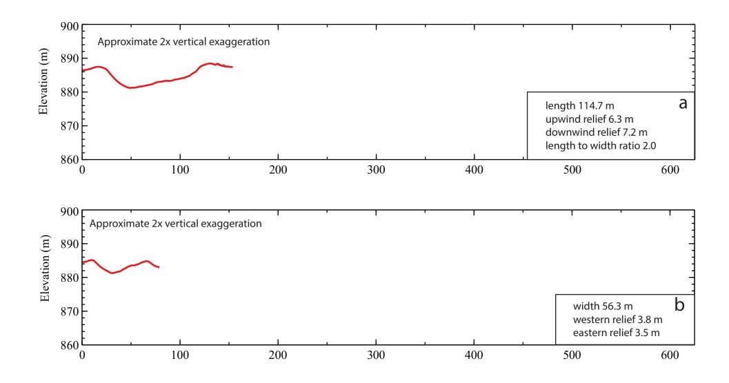
Supplementary Figure 4h. (a) Longitudinal profile of Conata Ranch Table polygon 12, upwind to downwind from left to right. (b) Transverse profile southwest to northeast from left to right. Approximately 2x vertical exaggeration.
