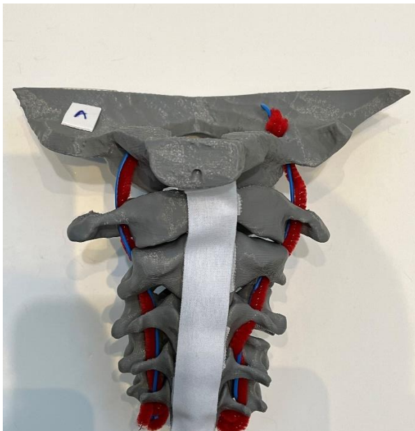
Figure 1. One of the 3D-printed cervical spine models. In this view, hook and loop fastener (white) is visible representing the anterior longitudinal ligament.
