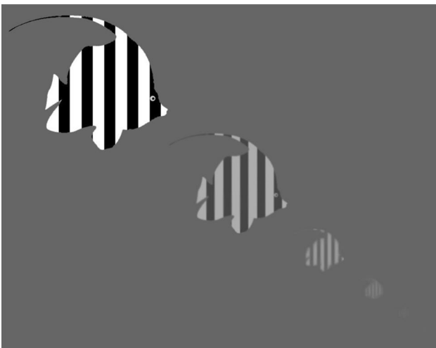
Fig. 2 The effect of viewing distance on the size, contrast, and sharpness of a patterned target. As the distance between the viewer and the target increases, the target becomes smaller, reduces in contrast due to path light, and loses fine spatial detail due to multiple scattering. At a certain maximal distance, the stripes are just barely discernible
