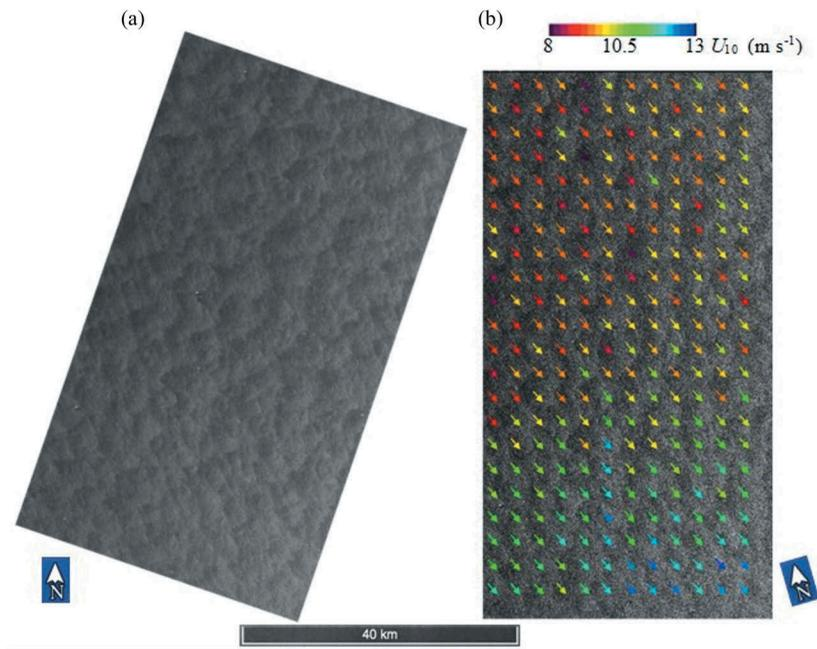
**Figure 2.** (a) The TerraSAR-X image acquired in VV on 10 February 2016 at 12:00 UTC, corresponding to the orange box in Figure 1. (b) The same TerraSAR-X image including spatial analysis of wind velocity. Wind speed is indicated by colour and vector direction.
