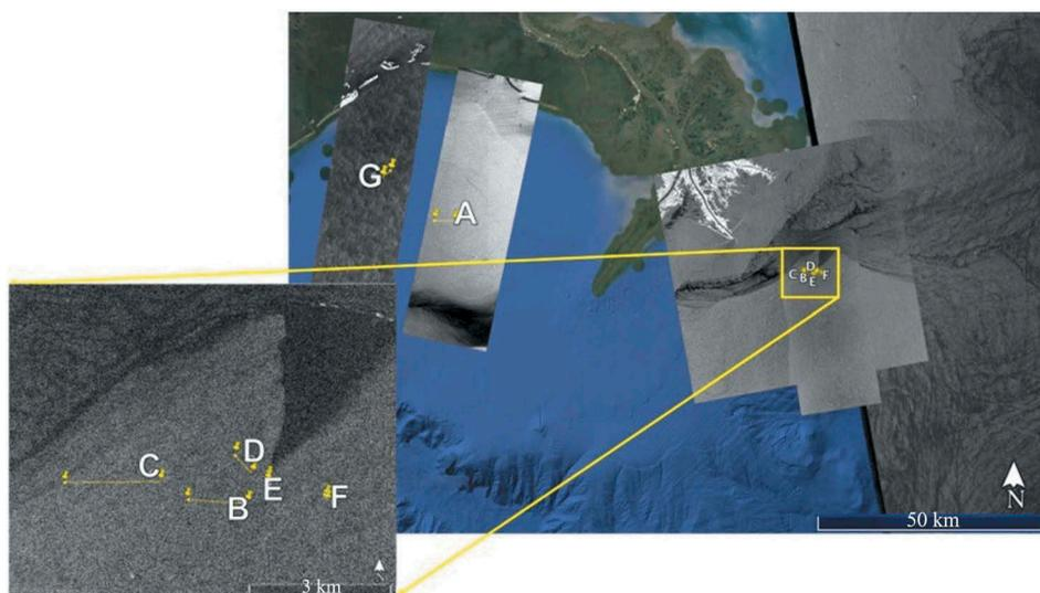
**Figure 4.** Sampling locations A-G from the SPLASH experiment in the Gulf of Mexico (Table 2). All SAR images taken over the course of the experiment are overlaid on the map. The small rectangular images are TerraSAR-X, the single square image is RADARSAT-2, and the largest image on the right side of the map is Sentinel-1.
