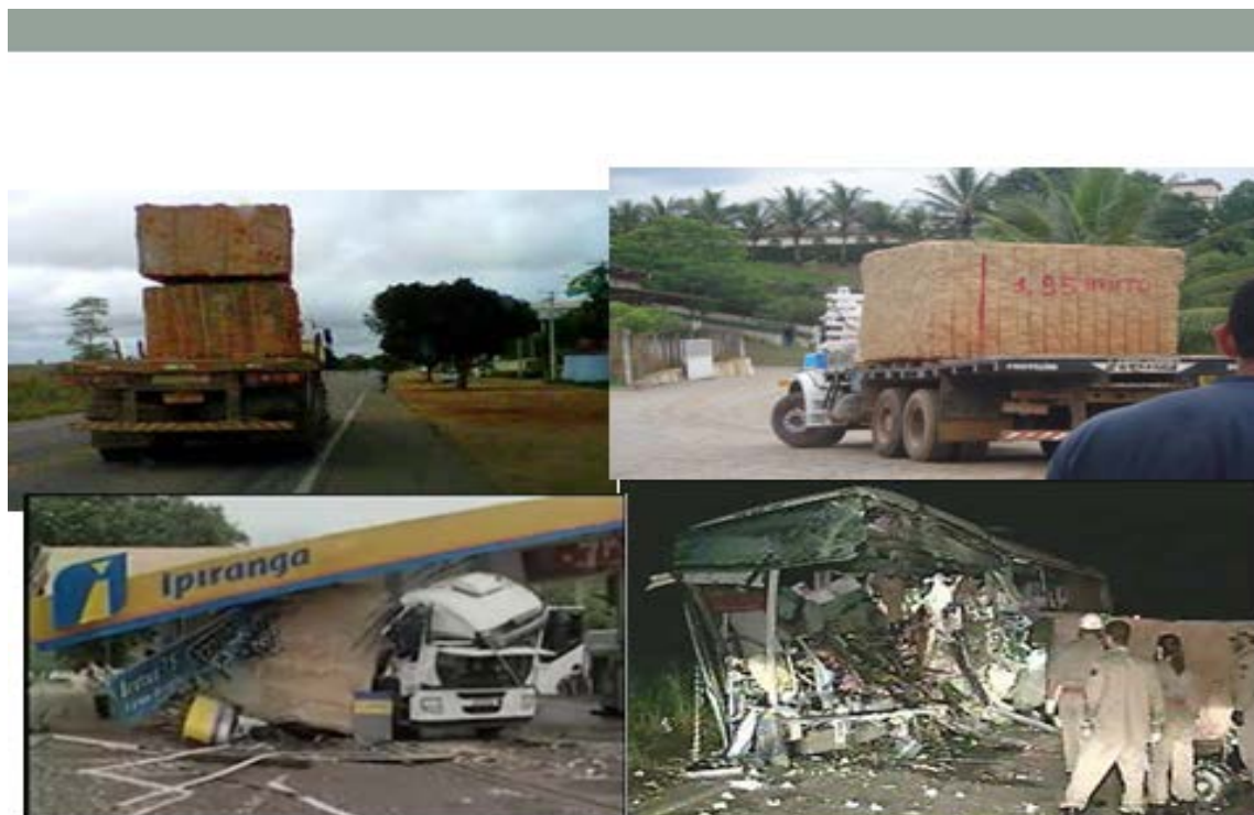
Figure 1. Granite blocks transported untied; accidents are caused by rock transportation.
