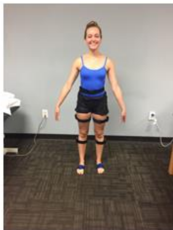
Figure 2. Setup of myoMOTION™ sensors in the neutral position that was assumed for calibration.
