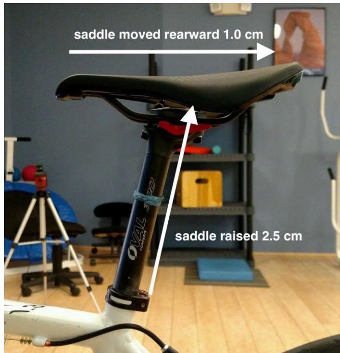
FIGURE 2. Saddle height and horizontal location adjustments
