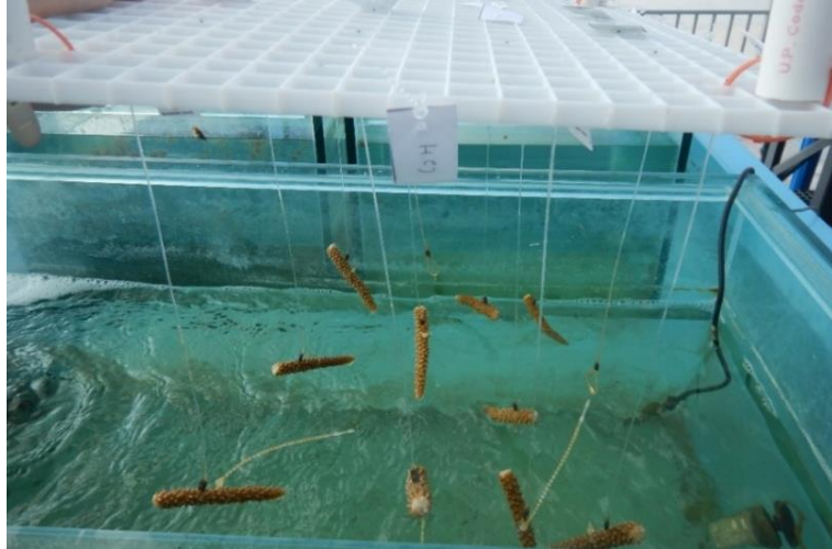
Figure 2. Experimental hanging design. Fragments were hung into tanks from egg crate using 12-inch long monofilament and crimps. Each fragment was spaced approximately 2.5 inches apart and the location of each fragment was randomized in each tank. The egg crate rested on the top of the tank and corals were suspended in the middle of water column.
