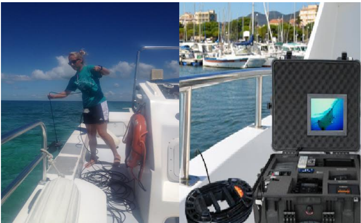
Figure 4. Drop camera video recorder setup
