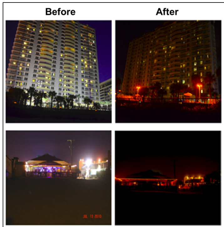
Figure 5 Before and after photographs of two commercial properties that incorporated sea turtle friendly lighting (STFL). (Adapted from Barshel, et al. 2014.)
