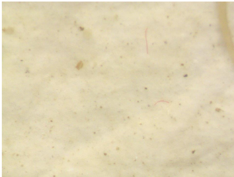
Photograph 4. Osprey 3129 GI Tract Filter: This is a photograph taken from one of the GI tract samples for the osprey 3129 filter. It is an example of microplastic fibers and how they may appear under the microscope, these fibers seen are of red coloration.
