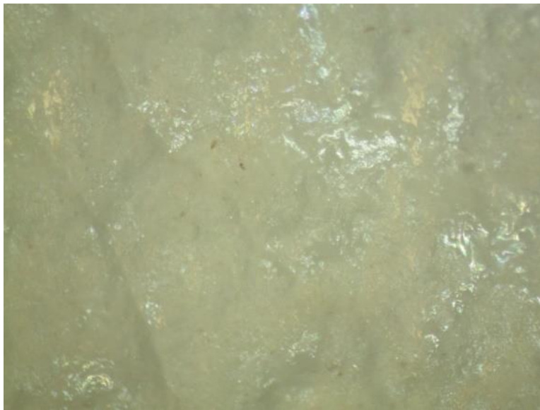
Photograph 2. Double-crested Cormorant 3219 Blank Filter: This is a photograph taken from the blank KOH sample for the Double- crested Cormorant 3219 filter. It is an example of the small unidentified particles found in many of the blank samples.
