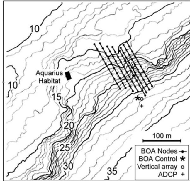
**Figure 5.** Array of instruments deployed at study site in Leichter et al. (2005) study.
