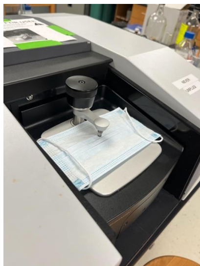
Figure 5: ATR-FTIR analysis of a blue surgical face mask at the NSU Main Campus.
