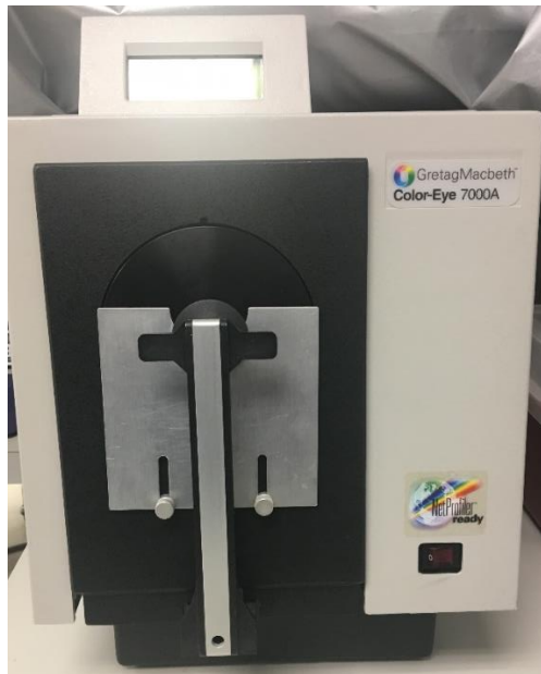
Figure 14. Scanning spectrophotometer (Color-Eye 7000A, Gretag Macbeth Instruments Corp., New Windsor, N.Y., USA).
