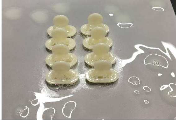
Figure 8. Samples printed with SLA printer with excess resin prior to cleaning.
