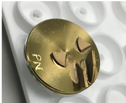
Figure 16. Specimens prepared for scanning electron microscopy.
