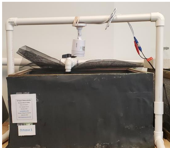
Figure 9: Camera Design for Food Preference and Associative Learning Experiments
