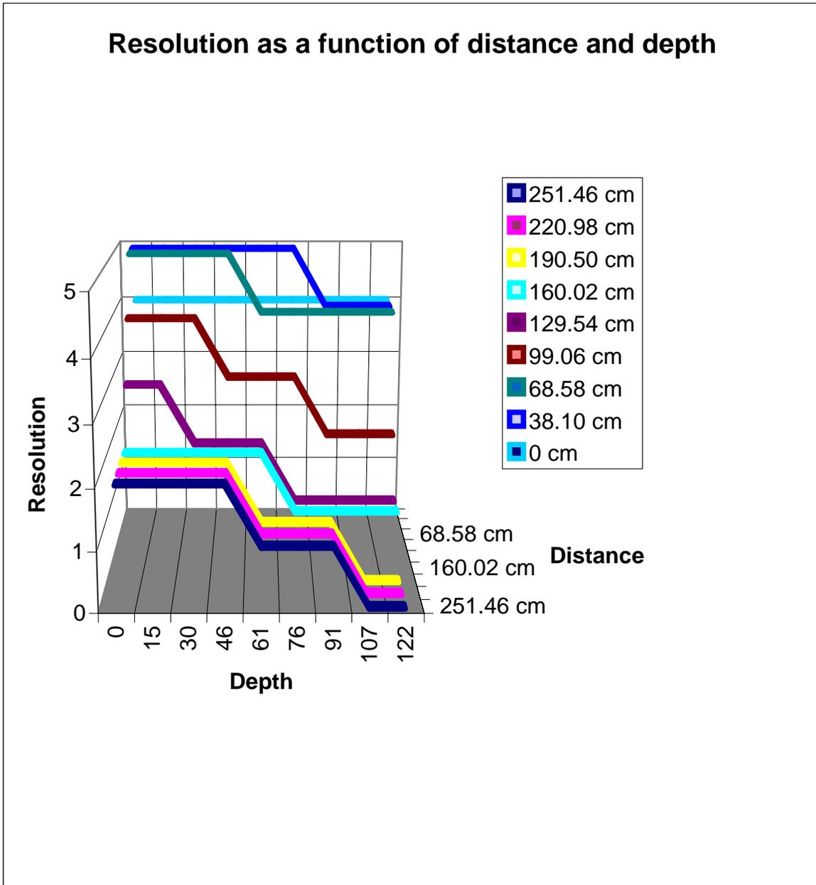
Figure 7. Resolution of the Atlantis Camera varied by distance and depth when using the sponge target. Note that generally this camera had greater resolution than the SeaView Camera.
