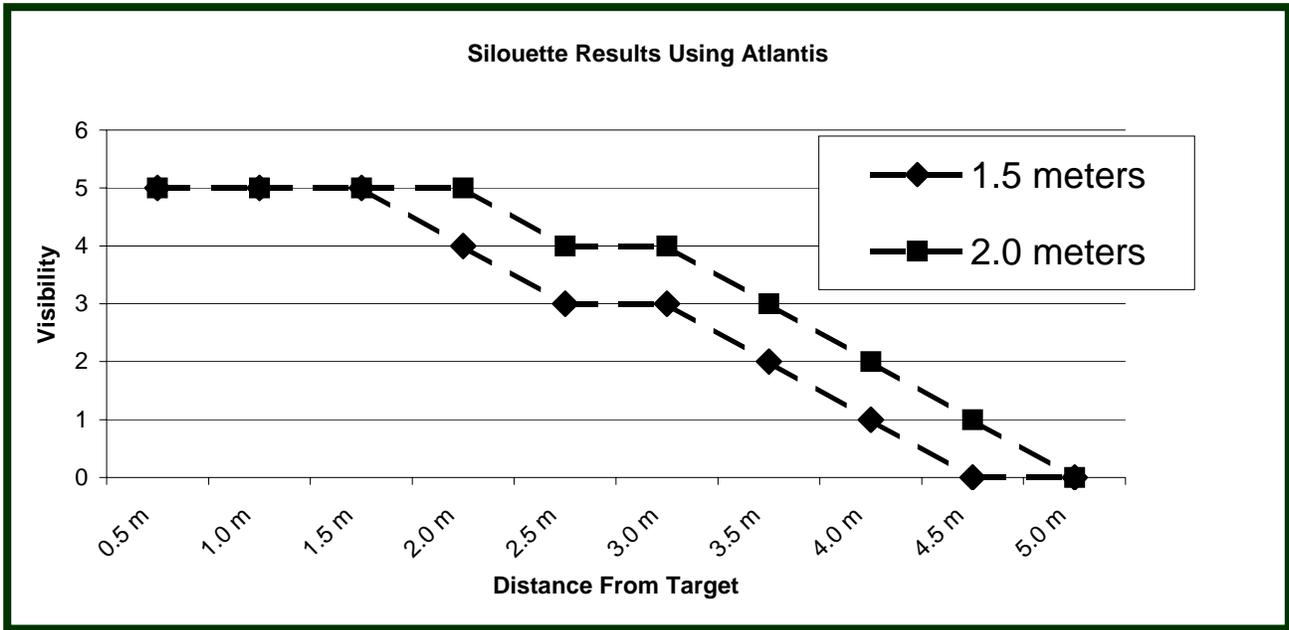
Figure 10. Quantification of the ability of the Atlantis camera to detect the plywood manatee silhouette at 1.5 and 2.0 meters depth.
