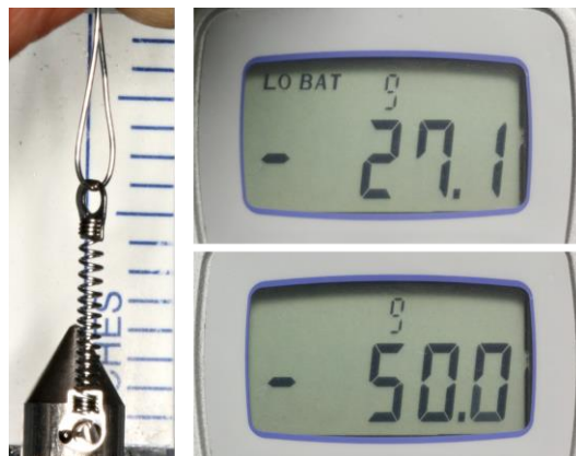
Figure 3: Force Gauge Measurements of the NiTi Spring used to apply orthodontic force.
