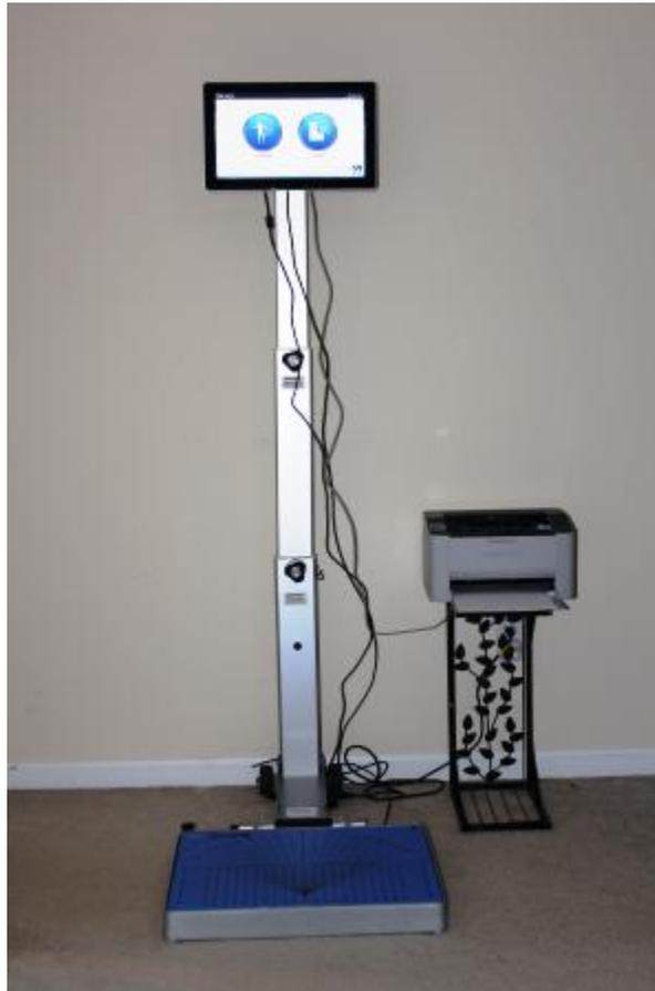
The Postural Stability test emphasizes a subject's ability to maintain center of balance. The subject's performance is noted as a stability index (in degrees from level) and it represents the variance of platform displacement in the forward, backward, left, and right directions.<sup>26,81</sup> The scores on this test assess deviations from the center, thus
