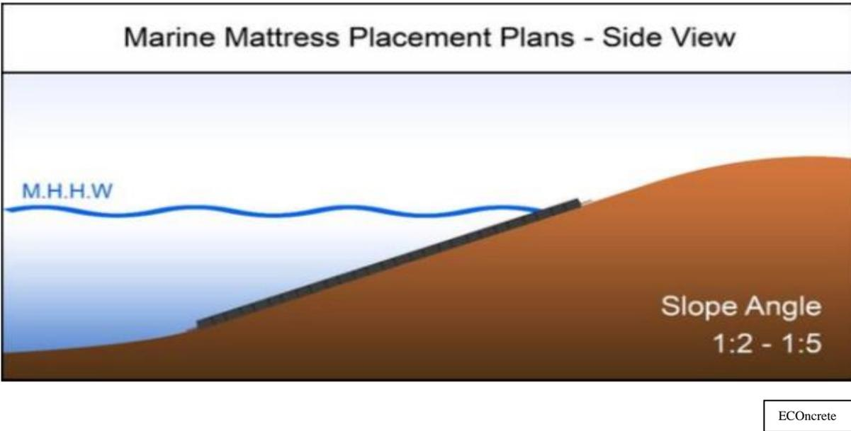
**Figure 5.** Side view of deploying ECONcrete® Articulated Concrete Block Mattress. Mean Higher High Water, (MHHW).
