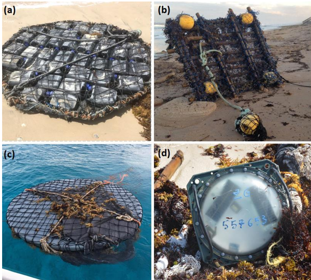
Figure 7. Photographic examples of common FAD components. The typical construction of an octagonal dFAD platform composed of 5L oil containers. Photo courtesy of Kelli Ann Briggs (a). A square bamboo dFAD platform wrapped in non-compliant net cover, photo courtesy of Thomas Pitchford (b). A Zunibal Zunfloat™ with a shade cloth and non-compliant net cover, photo courtesy of John Chamberlain (c). A Marine Instruments M3i+ satellite-linked beacon buoy with post-manufacturing markings stating “ZG 557653” in blue paint marker, photo courtesy of Raven Hoflund (d).
