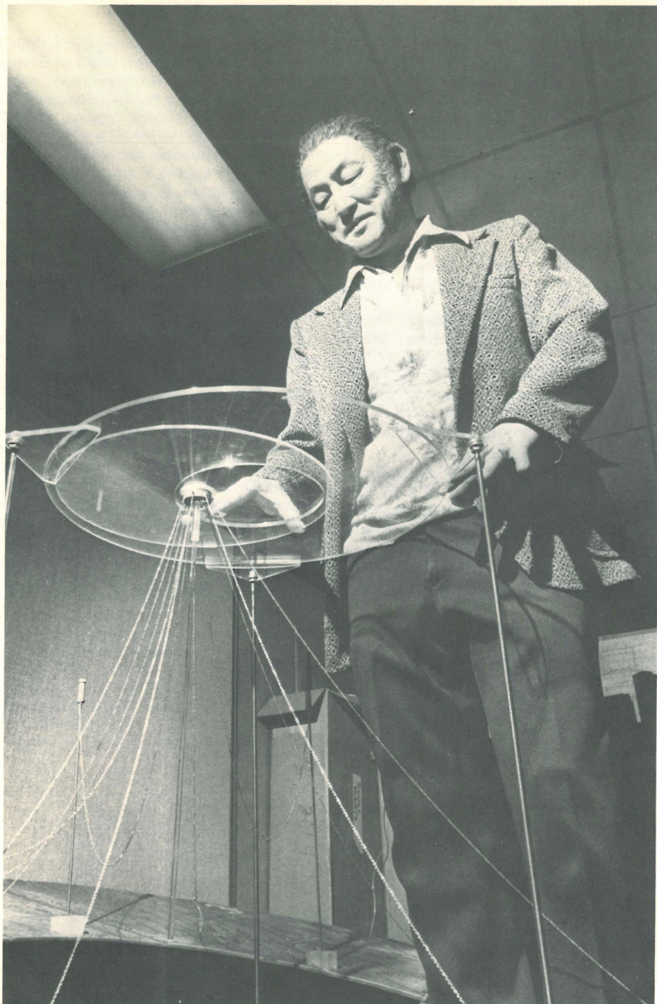
Lockheed senior naval architect Terry Iwashita displays the model of a mooring system for a large OTEC power plant developed under a DOE contract. Supported by three metal rods, the clear plastic represents the ocean surface and the drift circle of the OTEC plant moored in 4500 feet of water. Lines from the surface OTEC unit represent mooring and energy-transmission cables, which must function under widely varying sea conditions.
