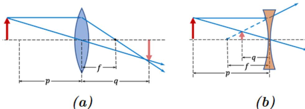
FIG. 1. (a) Converging and (b) diverging lenses.
