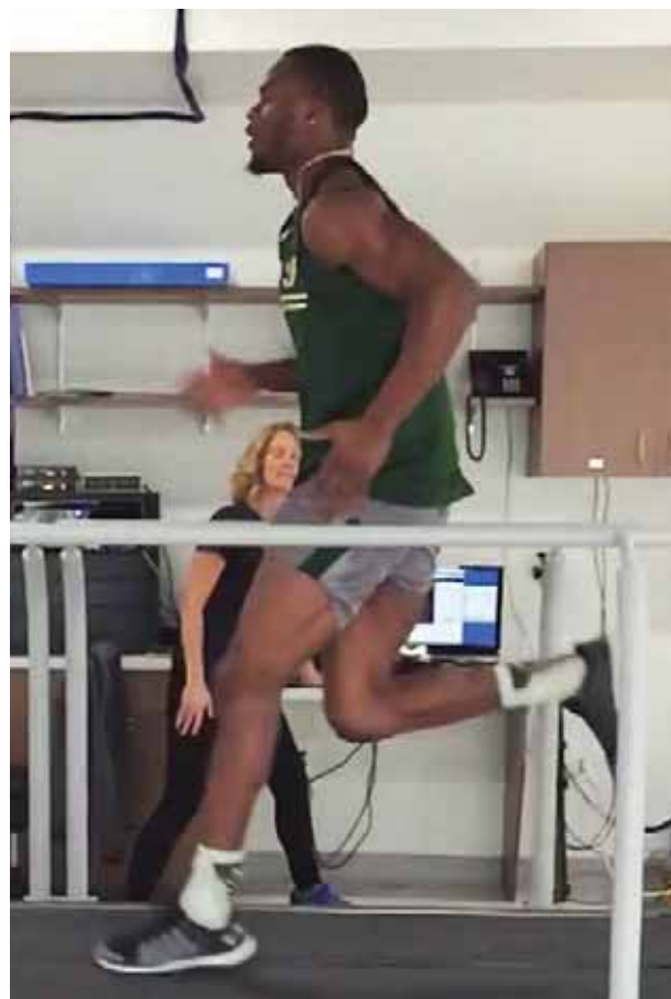
Right: A football player takes part in sub-max sprinting on the instrumented treadmill that measures forces.
