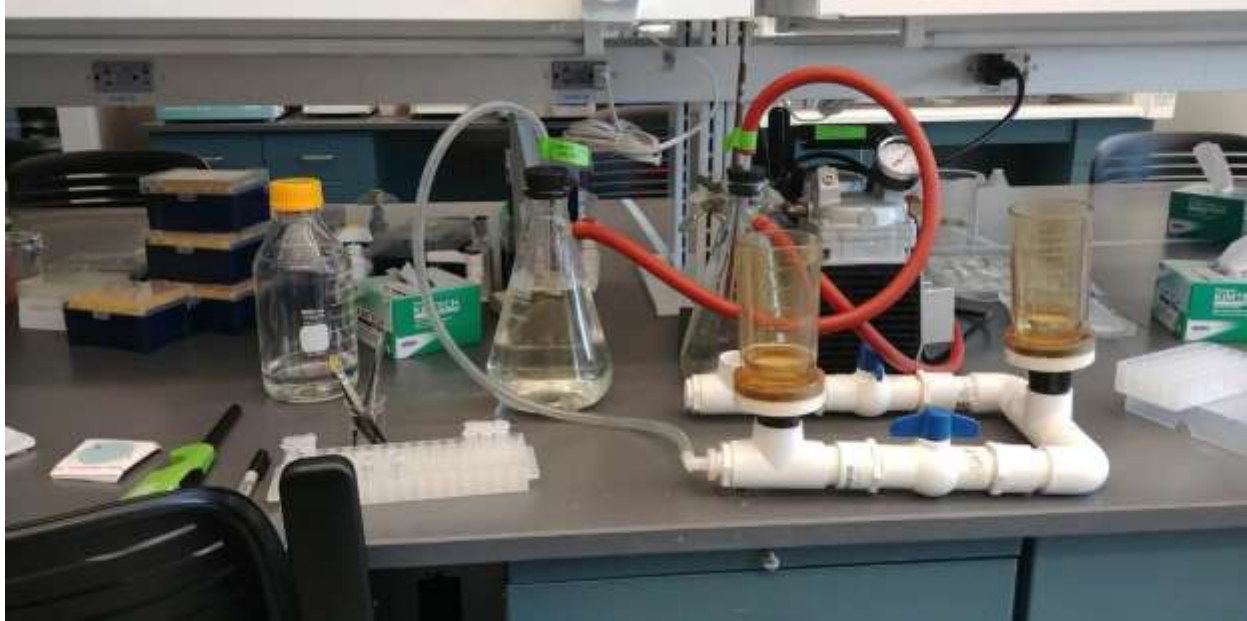
Figure 12: two 300ml magnetic filter funnels attached to PVC pipes hooked up to two filtering flasks and a vacuum pump
