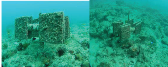
Figure 1. Settlement plate array design. Twelve arrays deployed to each of 5 sites for a period of one year.
