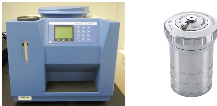
Figure 1. An IKA Bomb Calorimeter (C200si) equipment and vessel as used in this experiment.
