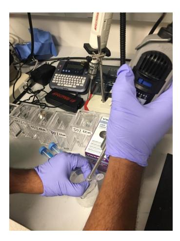
Appendix C:.Homogenizer tool used for HPLC protocol
