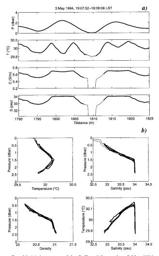
FIG. 16. (a) A segment of the *P*, *T*, and *S* record on 3 May 1994 at an intersection of the air–sea interface; (b) *T* and *S* as function of *P* and *T*–*S* diagram calculated from the segment shown in (a). Thin lines represent the raw signals, while the bold lines are the signals after processing.
