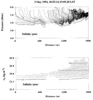
FIG. 15. Contour plots of *S* vs *P* and of *S* vs  $\sigma_t$  calculated during intersection of a surface freshwater lens (wind speed 2.7–4.6 m s<sup>-1</sup>, ship speed 2.4 m s<sup>-1</sup>).
