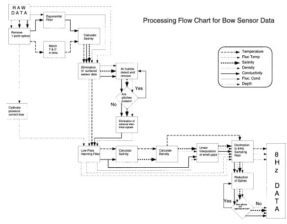
FIG. 9. Temperature and conductivity processing flowchart.
