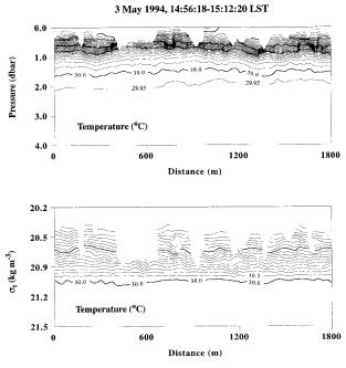
FIG. 14. Contour plots of *T* vs *P* and of *T* vs  $\sigma_t$  calculated during strong diurnal warming of the upper 1-m layer of the ocean (wind speed 2.2–2.4 m s<sup>-1</sup>, ship speed 2.0 m s<sup>-1</sup>).
