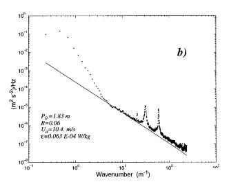
FIG. 11. (a) Spectrum of longitudinal  $(V_x)$  fluctuation velocity (dashes) in comparison to spectrum of integrated longitudinal  $(g_x)$  acceleration (solid line). (b) Wavenumber  $V_x$  spectrum (points) and theoretical spectrum of turbulence in inertial subrange. Ship speed is 10.3 kt.
