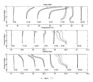
FIG. 13. Vertical profiles of temperature, salinity, and density obtained by averaging 10-min intervals of the bow sensors' data within 0.1-db pressure ranges. Each successive profile is shifted by 1°C in temperature, by 0.5 psu in salinity, and by 1.0 kg m<sup>-3</sup> in  $\sigma_i$ . The time below each profile corresponds to the middle of the 10-min segment. Thin lines represent ±1 std dev.
