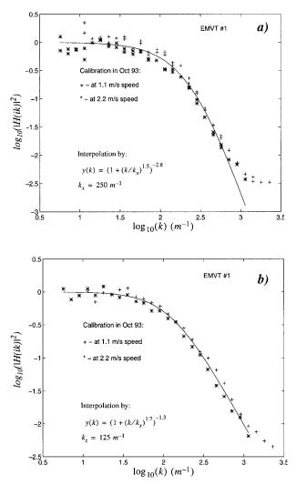
FIG. 8. Spatial response for (a)  $V_x$  and (b)  $V_z$  channels. Here |H(ik)| is the wavenumber response-function magnitude, k is the radian wavenumber ( $k = 2\pi/\lambda$ , where  $\lambda$  is the wavelength in meters per cycle), and  $i^2 = -1$ .
