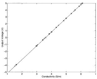
FIG. 7. Comparison of conductivity calibrations for ECTP #1 made in Granit and at JHU/APL; "O" denotes calibration points obtained in Granit; the straight line is their regression. "\*" and "+" denotes calibration points measured by JHU/APL on 19 and 23 May 1995, respectively.
