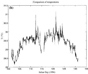
FIG. 10. Comparison of the bow and thermosalinograph temperatures and salinities. (a) Bounds of the observed depth range of the bow sensors measurements (contiguous straight line represents 2.9m depth and dashed line represents the 4.4-m depth); (b) bow (dots) and thermosalinograph (thermistor at bow intake) temperatures (solid curve), and (c) bow (dots) and thermosalinograph (solid curve) salinities.
