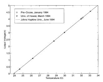
FIG. 6. Comparison of temperature calibrations and tests of ECTP #1; "o" denotes the calibration points obtained in Granit by thermometer with 0.01°C accuracy; "\*" denotes the points obtained during testing at the University of Hawaii; straight line is the regression estimated by JHU/APL from the JHU/APL calibration data.
