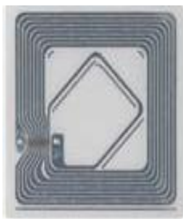
Figure 1. Basic 3M™ radio frequency identification (RFID) book tag used for typical library implementations (actual size). Photo of 3M product reprinted with permission.
