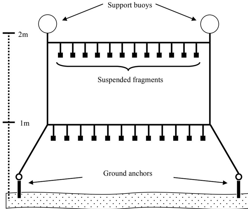
Figure 41. Diagram of suspended nursery module showing the position of suspended fragments in this study.
