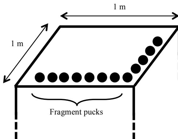
Figure 40: Diagram of a concrete nursery module and the placement of pucks. Not to scale; actual puck capacity 36 (module surface perimeter able to accommodate four rows of nine pucks).
