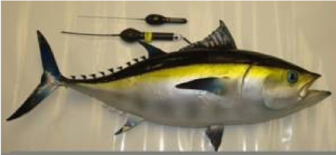
Figure 2: Relative sizes of Microwave Telemetry, Inc. X-Tag (top) and standard model (bottom) pop-up satellite archival tags (PSATs) next to a 72 cm fork-length mount of a blackfin tuna ( Thunnus atlanticus ). The targeted swordfish individuals will be less than 150 cm lower jaw-fork length. (Photo courtesy D. Kerstetter, NSU OC)
