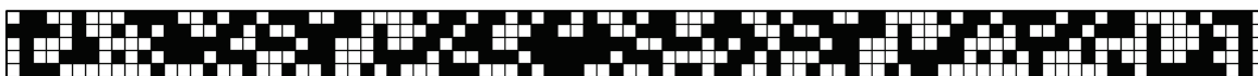
Figure 1. Operation of cellular automaton rule 1205312089 with the first 96 bits of data from packet 1,819 of the Friday week two training data. The initial data and four cycles of the cellular automaton cell values are shown as five rows in the figure. The ones density does not decrease below the density threshold for this rule. This packet would not be selected as a match.
