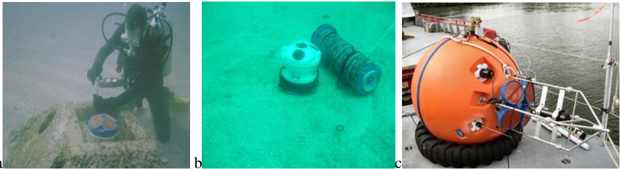
Figure 2. Photographs of the ADCP Bottom Mount (a), AWAC Bottom Mount with battery on the right (b) and Calypso subsurface buoy on the deck of the towboat Becker (c).
