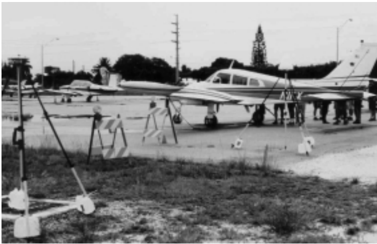
NASA plane used for flying EAARL Lidar with GPS ground station in foreground.
