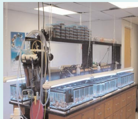
Experimental corals collected off Fort Lauderdale, and placed in 2.5-gallon aquaria. Treated colonies received carbonate sand (<500 mm) rate of approximately 150 \text{ mg/cm}^2/\text{day} during the five-week period.
