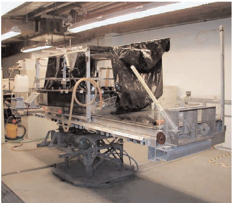
Turntable used in the laboratory experiments (Arizona State University, Environmental Fluid Dynamics Program). The tank diameter is approximately 2m. The apparatus is covered by plastic during the experiments to avoid the adverse effect of wind stress.
