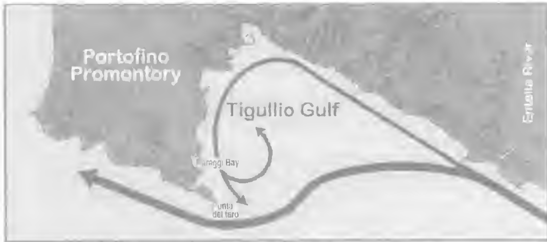
FIG. 1. Schematic figure showing the main current patterns in the studied area. At Punta del Faro, the current from the Golfo Tigullio meets the main cyclonic stream of the Ligurian Sea. Paraggi Bay represents a decantation area consequent to an eddy.
